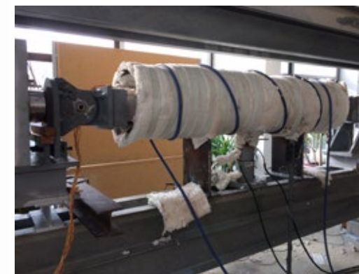
Laboratory unit for testing load-bearing elements in high-temperature conditions
